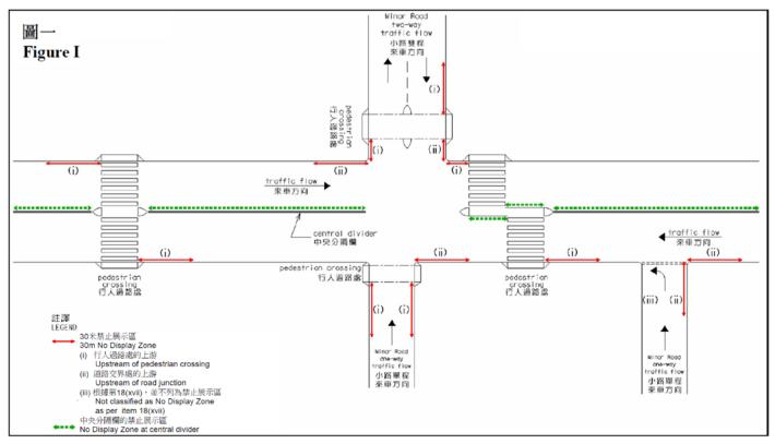
A plan illustrating the requirements of subparagraphs (vii) to (ix) is at Figure I.
